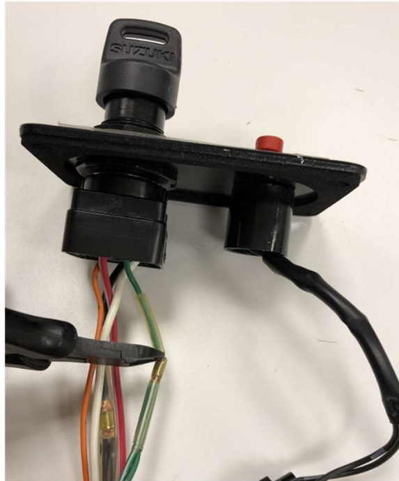
Key switch with one green wire
