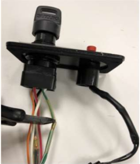
Key switch with one green wire
