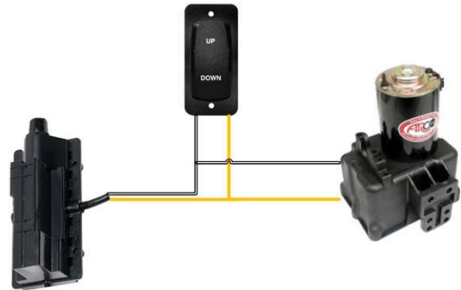
Figure 4 - Circuit for additional functions (Optional)
